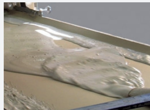
Gypsum wallboard production line: High potential of water reduction with use of Sika® ViscoCrete® G-2
