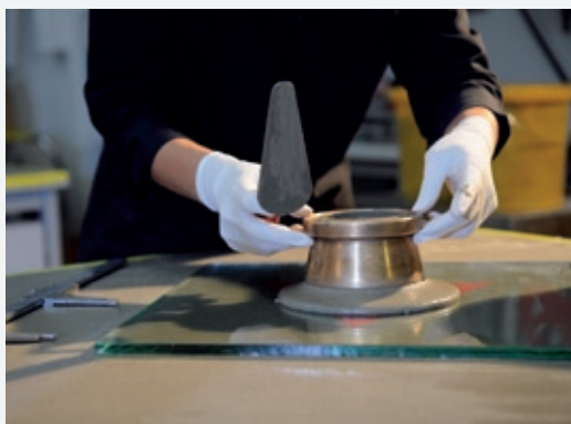
Admixture performance test in Sika's Technology Center
